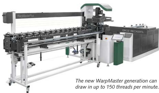
*The new WarpMaster generation can draw in up to 150 threads per minute.*
