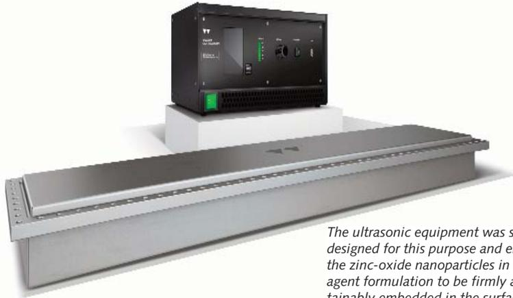
*The ultrasonic equipment was specially designed for this purpose and enables the zinc-oxide nanoparticles in the active agent formulation to be firmly and sustainably embedded in the surface of all kinds of textiles, with lasting effect. Image source: Weber Ultrasonics AG.*
