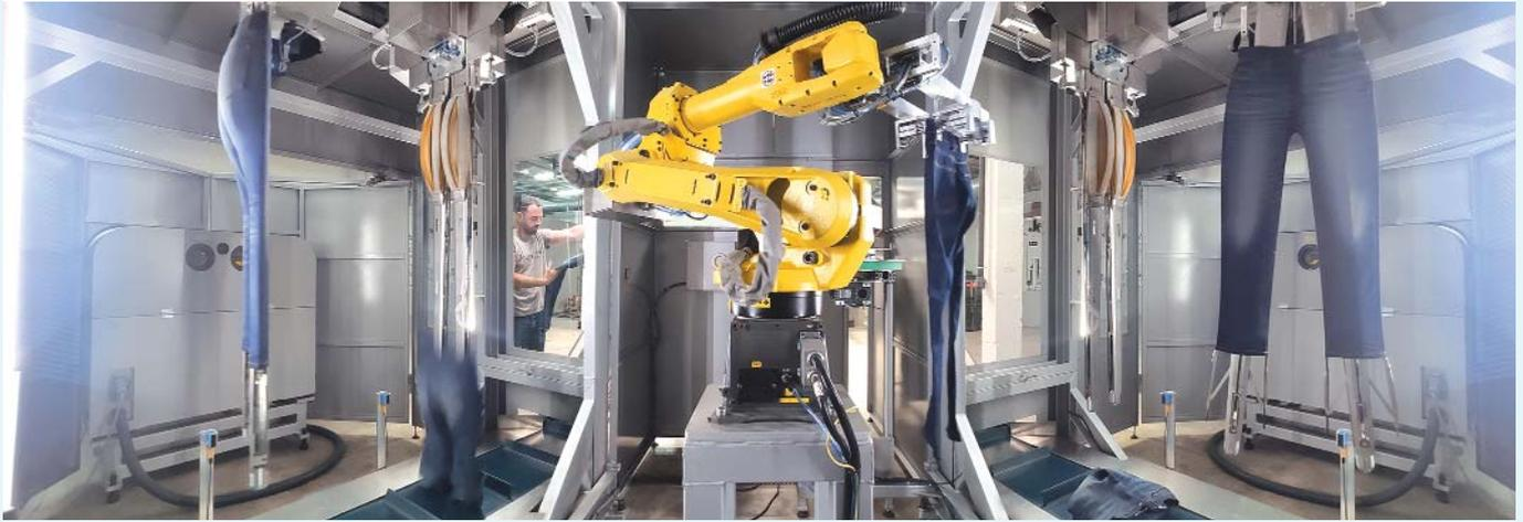
The technology is equipped by two lasers and a robot cabinet. A human and a robot work together to produce with scalability, agility, sustainability, and efficiency. Two humans working with two robots can produce 10,000 vintage jeans in 24 hours without discharge. Handman is a reality and currently is in use in 3 plants around the world, producing 5 million jeans a year.
