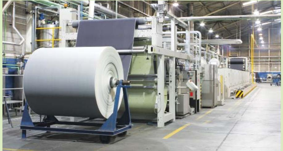
Monforts has a leading position in the field of denim finishing with its well proven Thermex continuous dyeing systems, Montex stenter dryers and other lines for resource-efficient and economical processing.
