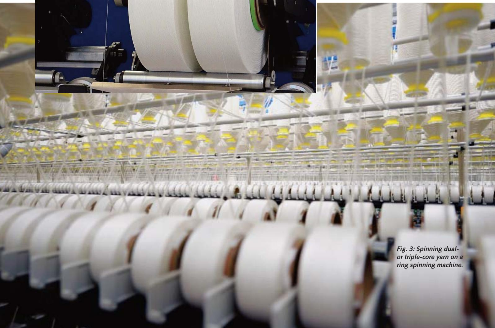
*Fig. 3: Spinning dual- or triple-core yarn on a ring spinning machine.*
