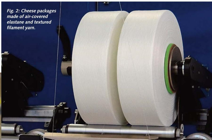
*Fig. 2: Cheese packages made of air-covered elastane and textured filament yarn.*
