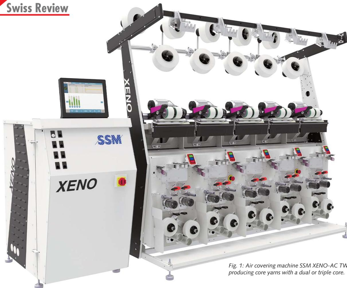
Fig. 1: Air covering machine SSM XENO-AC TWIN for producing core yarns with a dual or triple core.
