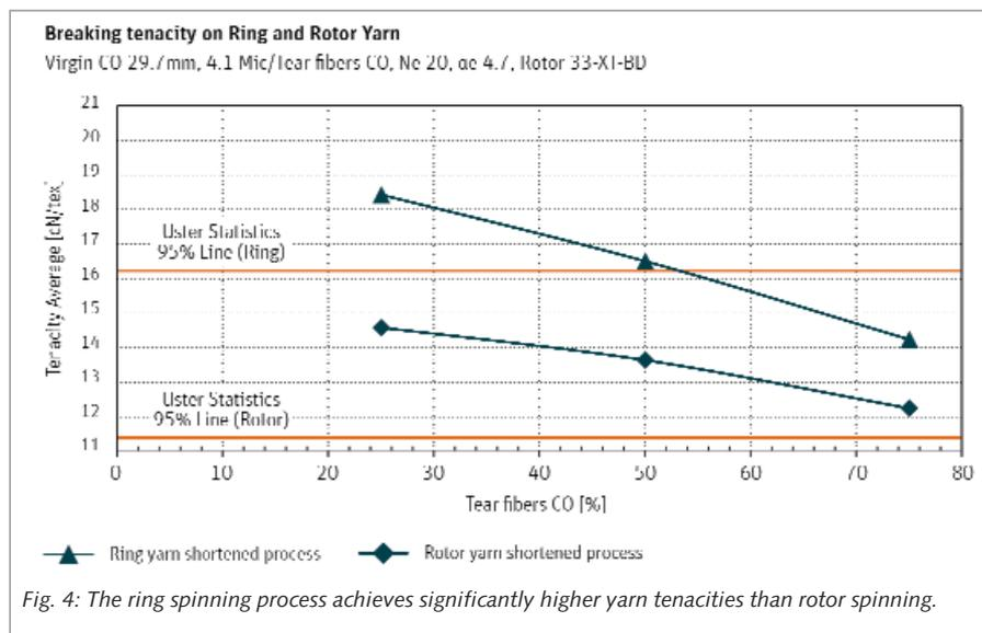
Fig. 4: The ring spinning process achieves significantly higher yarn tenacities than rotor spinning.
