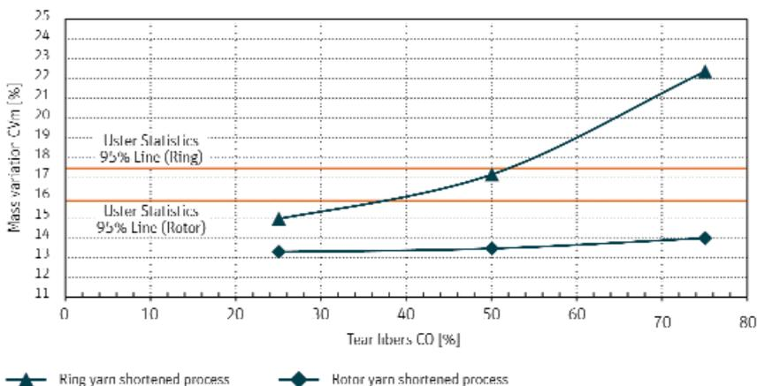
Fig. 3: The rotor spinning machine is well suited for processing fibers with a high short-fiber content, which is reflected in better evenness.
