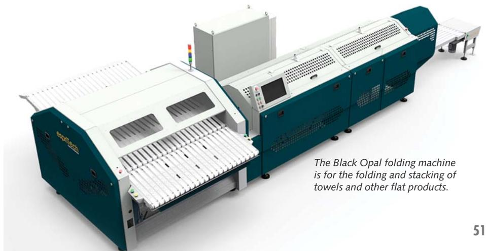
The Black Opal folding machine is for the folding and stacking of towels and other flat products.
