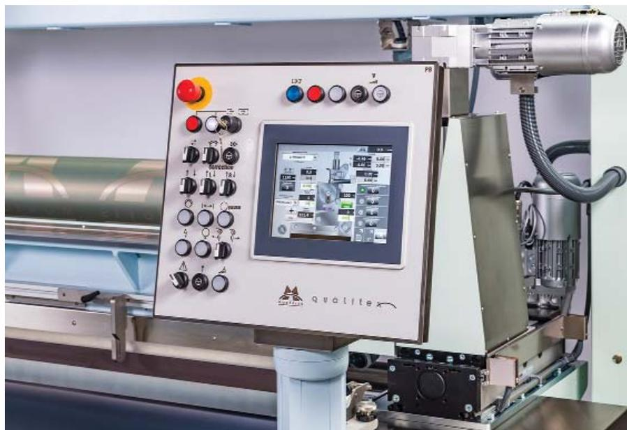
The touchscreen control of the Montex® Coat allows simple and easy adjustment of previously complicated settings.
