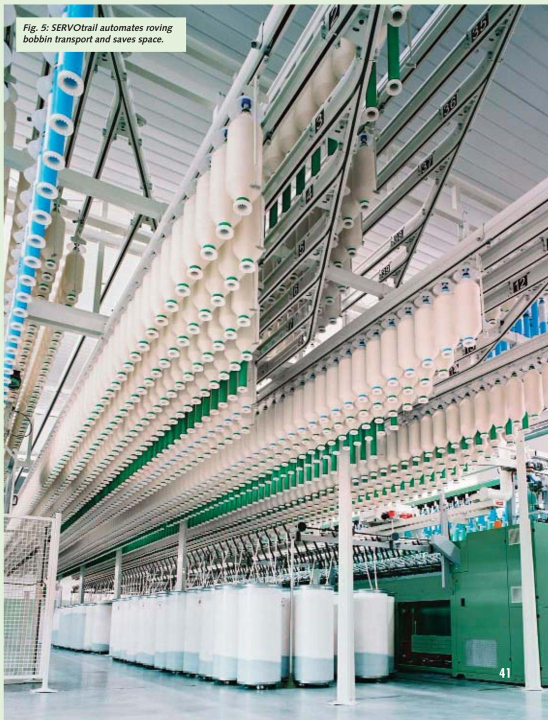
Additionally, SERVOrail saves space, ensures free access to the spinning machines, and improves the ergonomic handling of the roving bobbins (Fig. 5). The automatic transport system ensures that the roving on the bobbins is not touched. A consistently good roving quality is guaranteed.
