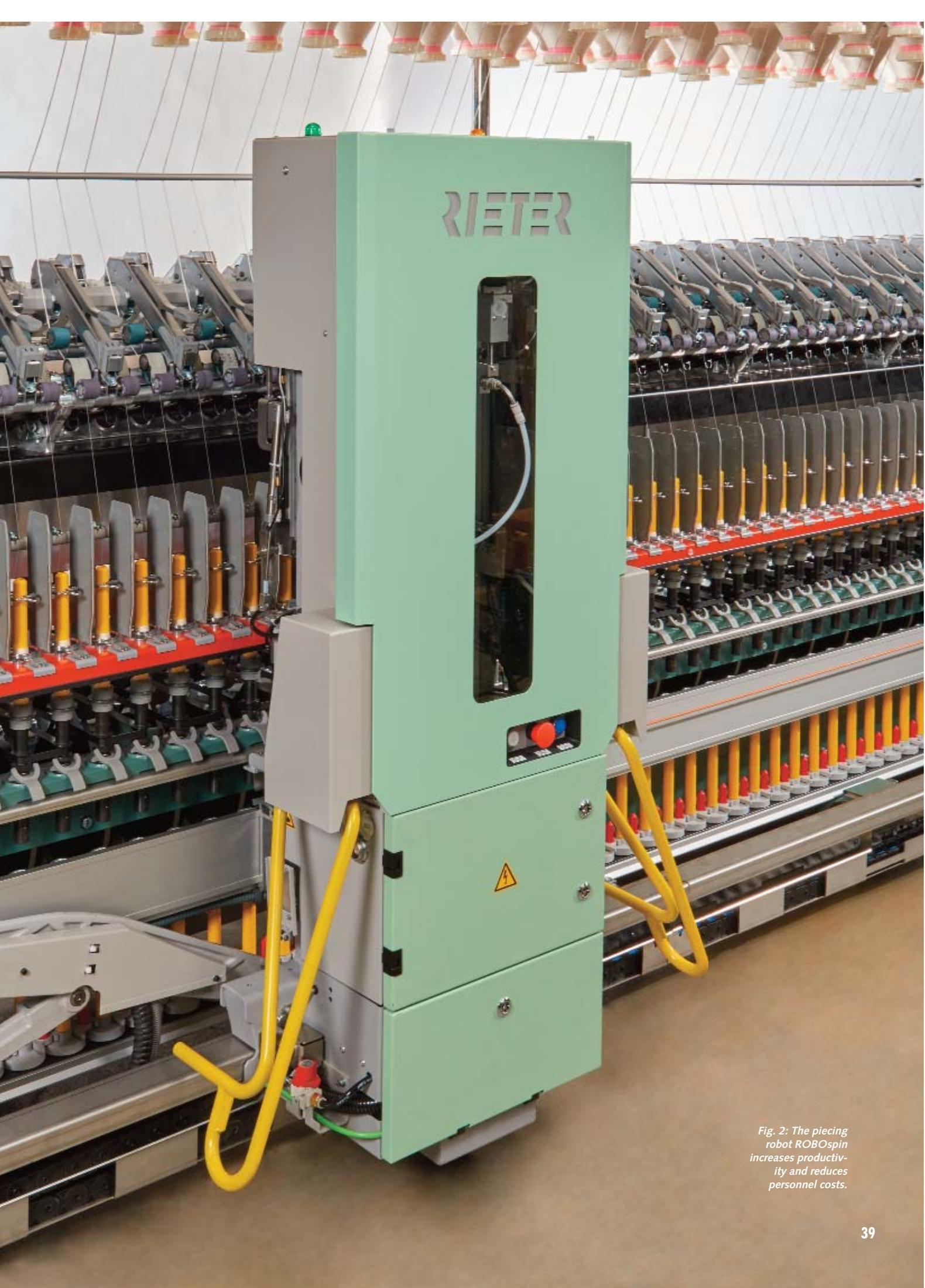
*Fig. 2: The piecing robot ROBospin increases productivity and reduces personnel costs.*
