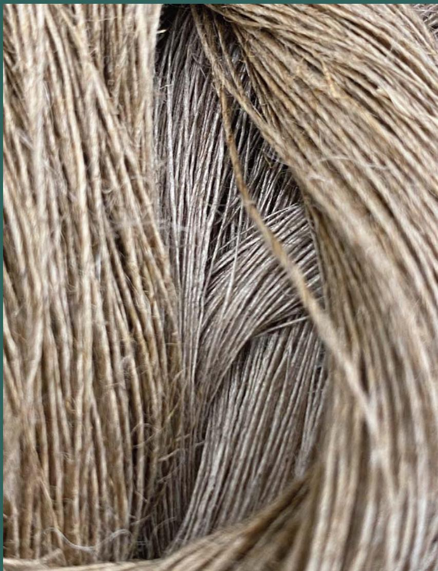
*Cottonization, is necessary to make the fibre suitable for spinning, because compared to cotton, hemp is longer, stiffer, and less flexible. © Cone Denim.*
