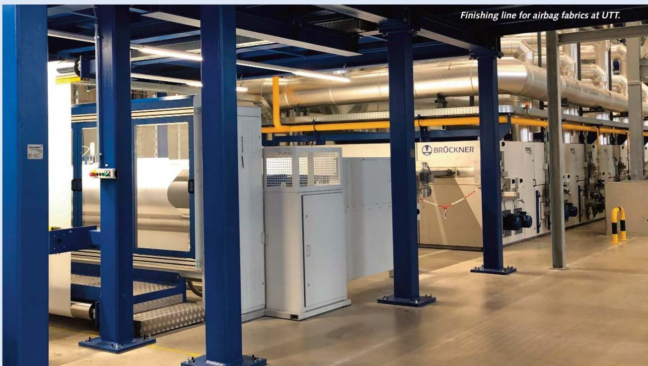
Finishing line for airbag fabrics at UTT.
