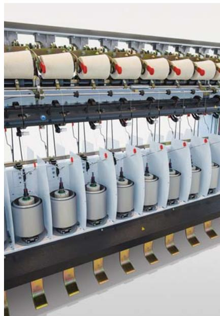
*FusionTwister spindle section.*
