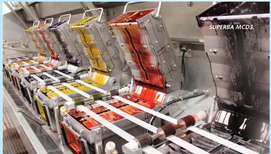
technology, the space-dyeing process has been renewed and undergoes a new boom. This technology enables to get yarn directly usable in carpet and rugs to realize innovative design. It is now possible to obtain up to 15 different color shades on the same yarn in one single working pass.
