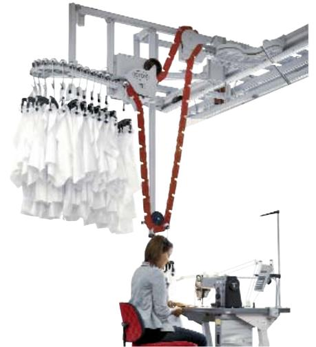
*Multiple rails enable rapid sorting at individual workstations.*
