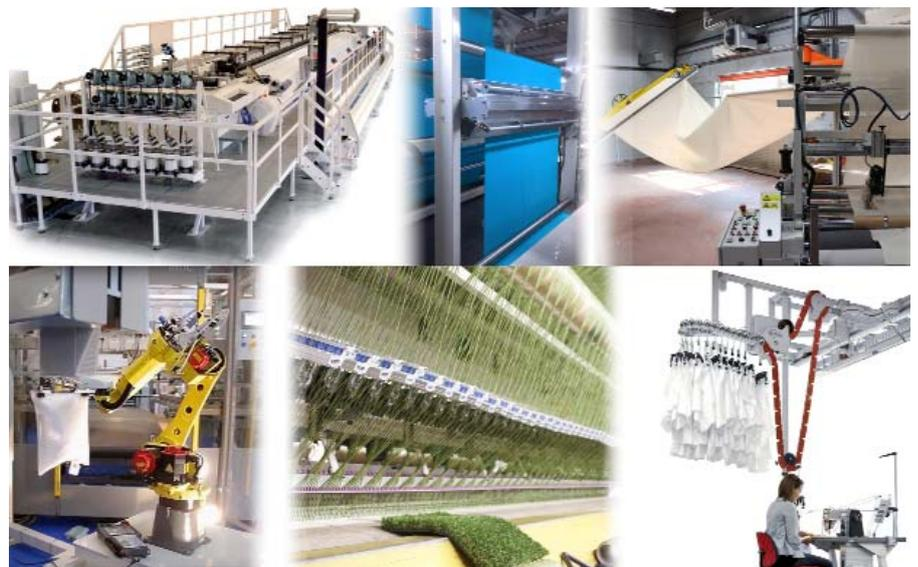
Some of the TMAS innovations to be introduced at ITMA 2019 (clockwise from top left) – Texo AB wide-width weaving technology, Baldwin’s new TexCoat G4, the latest bias cutting system for technical textiles from Svegea, Eton’s advanced material handling solutions, the Eltex EYE yarn fault detection system on a synthetic grass line, and robotic handling from ACG Kinna.
