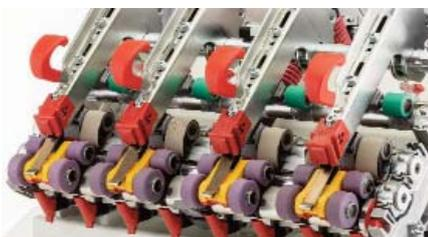
with new geometry of the compacting zone. Lattice apron 5star®BL improving wear resistance up to 20% hence longer lifetime and single suction tube type Pelican for less choking and easy cleaning and increased lifetime of EliTop cots up to 100% and reducing handling in buffing and workshop up to 50% and the EliSpring reduces end breaks up to 50%.
