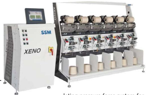
lating pressure force system for SSM XENO platform and **powerblade™**: New SSM XENO-PB, combines the advantages of blade winding and electronic yarn traverse. ♦
