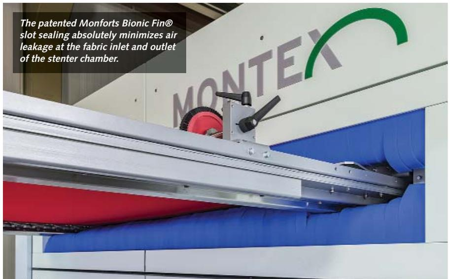
*The patented Monforts Bionic Fin® slot sealing absolutely minimizes air leakage at the fabric inlet and outlet of the stenter chamber.*
