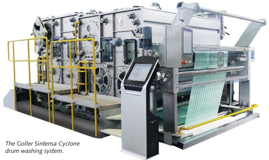
*The Goller Sintensa Cyclone drum washing system.*
