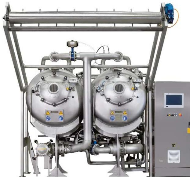
*The new THEN Supratec LTM hydraulic long tube dyeing machine.*
