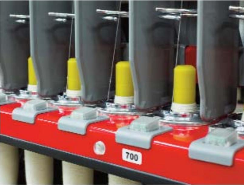
Fig. 2: The premium version of the individual spindle monitoring (ISM) is incorporated into the models G 38 and K 48. This reduces personnel requirements.
