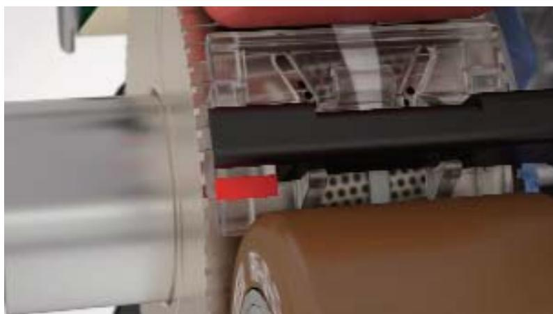
Fig. 4: The air guide element Detect for the compact-spinning machines ensures consistently high yarn quality.
