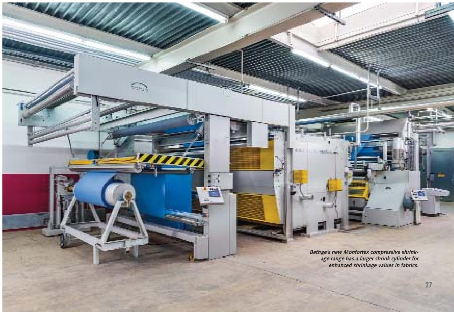
*Bethge's new Monfortex compressive shrinkage range has a larger shrink cylinder for enhanced shrinkage values in fabrics.*
