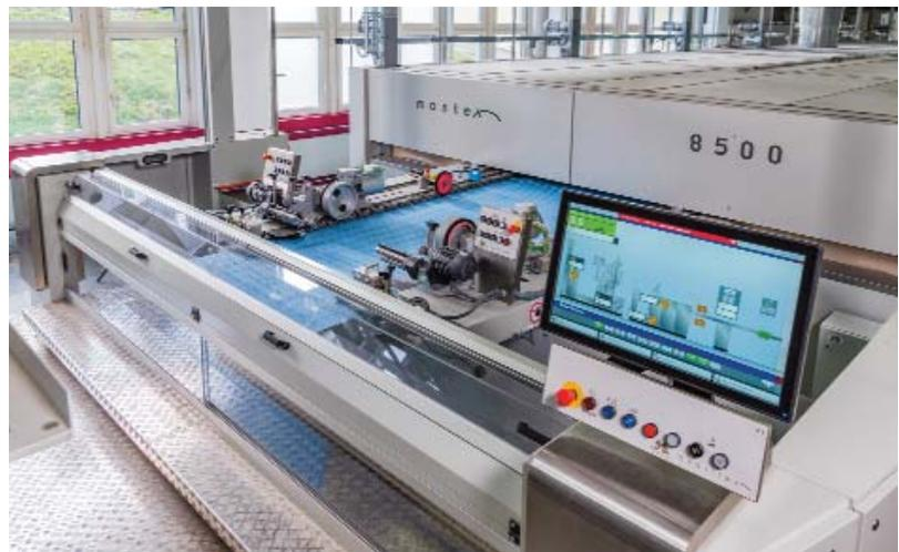
Intuitive automation and surveillance of the machines is via the Monforts Qualitex 800 control system.
