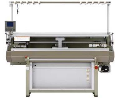
The World's First Digital Stitch Device, the Digital Stitch Control System(DSCS) can be programmed with the desired loop length, after which it monitors yarn consumption continuously and adjusts yarn feed and tension to yield consistency throughout the fabric to within a remarkable  $\pm 1\%$  tolerance. The result is quality control that is essential to shaping and integral garment production.
