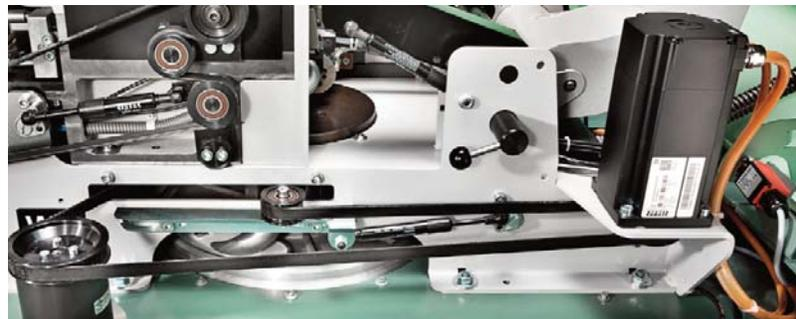
Fig. 2: The servomotor for the coiler allows rapid optimization of the speed.
