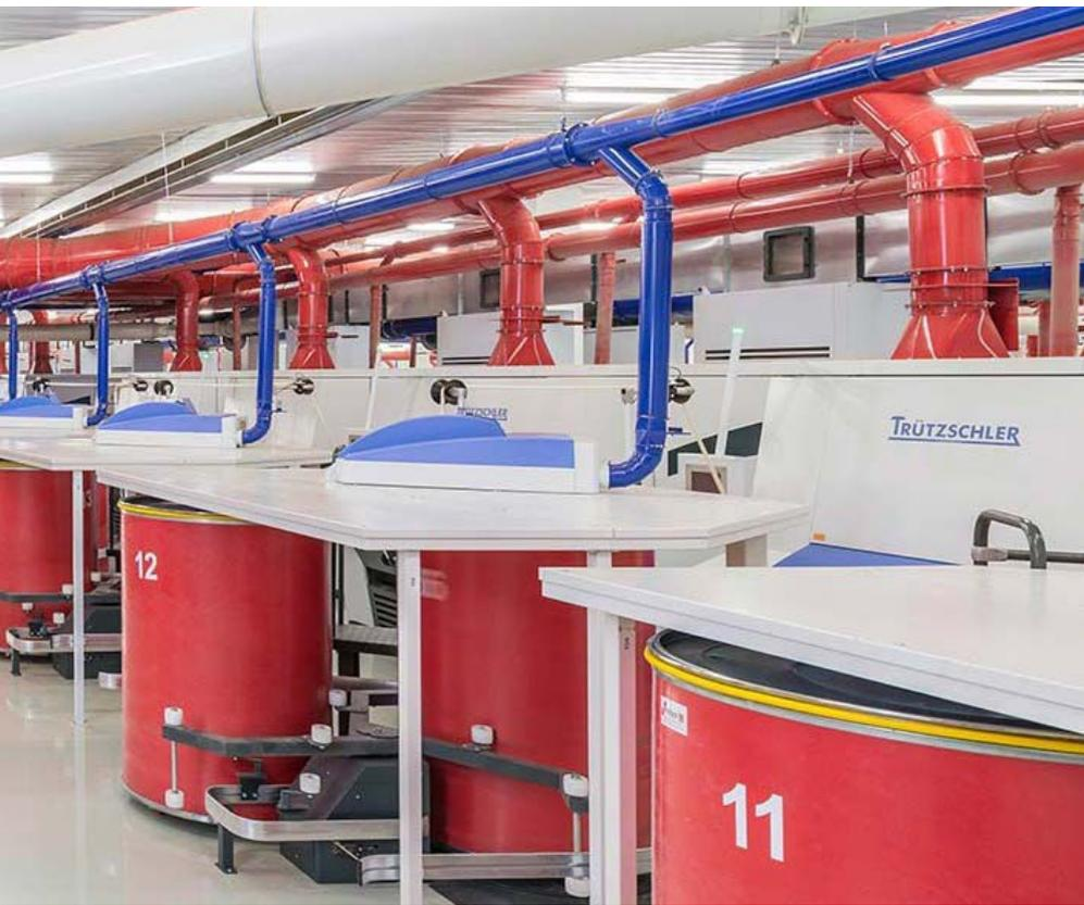
new sliver preparation technology. When processing viscose, two of three draw frame passages can be eliminated. This represents an enormous economic advantage.
