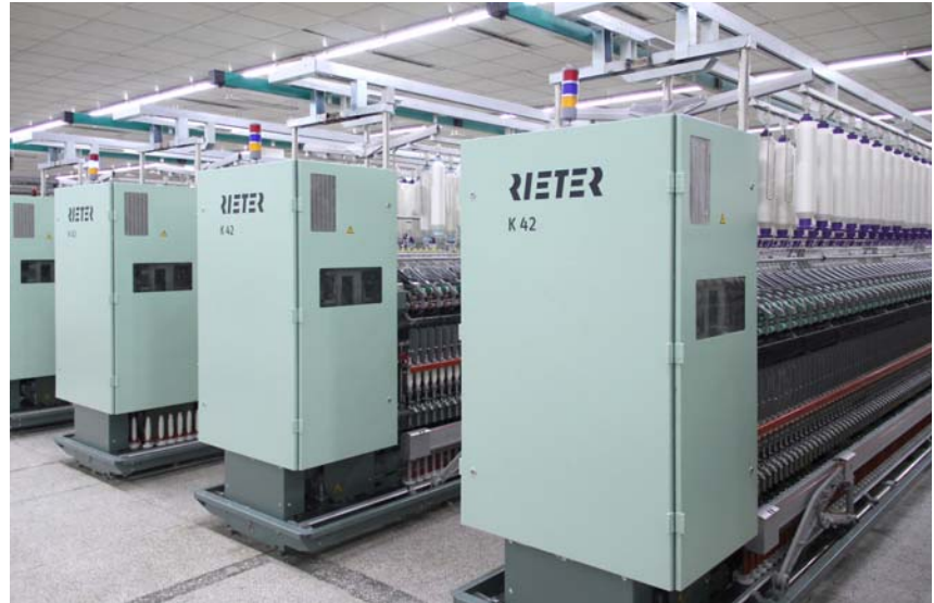
Fig. 1: The compact-spinning machine K 42 can achieve better results than those currently being achieved in China.
