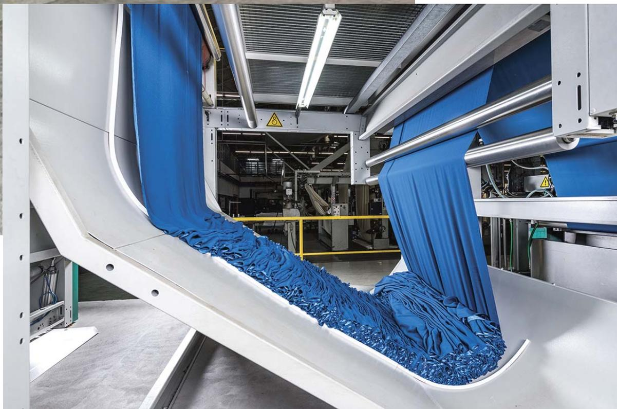
Special J-boxes at the Montex stenter's inlet and outlet allow for the gentle storage of a high volume of material.
