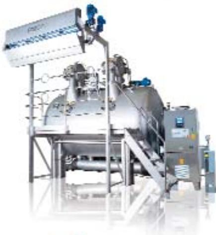
Optional blower for front misting spray nozzle to enhance the effectiveness of dye liquor interchange for more level dyeing effect!
