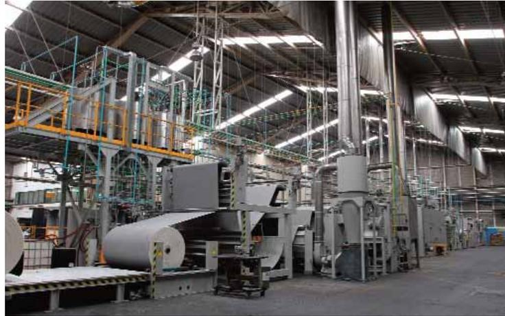
The new ThermoStretch skewing unit from Monforts offers new and improved features for Eco friendly denim finishing avoiding the excessive use of 'expensive to generate' steam that was previously necessary for the cylinder dryers; thereby replacing the need for steam-operated cylinder dryers.
