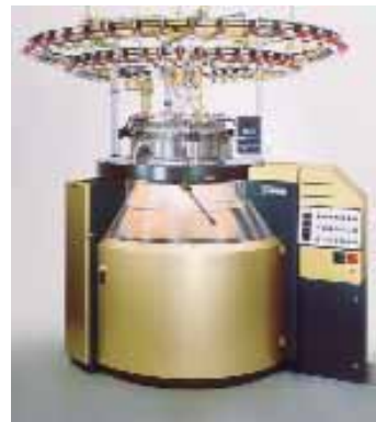
This is how a Relanit looked 30 years ago: Relanit 4, one of the machines presented on ITMA in 1987, works with four needle tracks.
