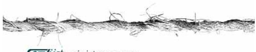
Com4jet – air-jet-spun yarn
