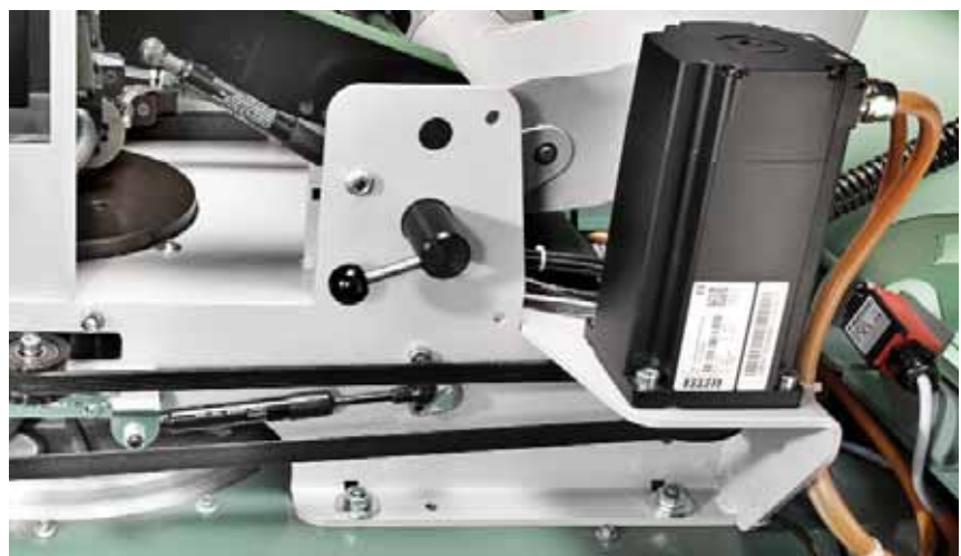
Fig.2: The servomotor for the coiler allows rapid optimization of the speed.
