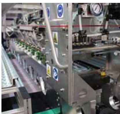
Since the printing heads on the MS LaRio are fixed, there can be no loss of alignment as the ink is dispensed, which helps eliminate printing errors.
