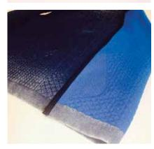
The new project concerns the knitting of an innovative denim double-face quilted fabric produced by Santoni's Double Jersey circular knitting machine the Mec-mor CMP and Lenzing's TENCEL® fiber.
