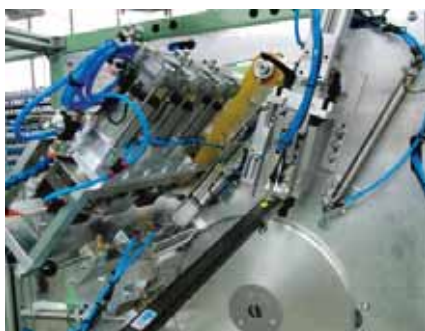
UV60-W – Tool changer and winder.
