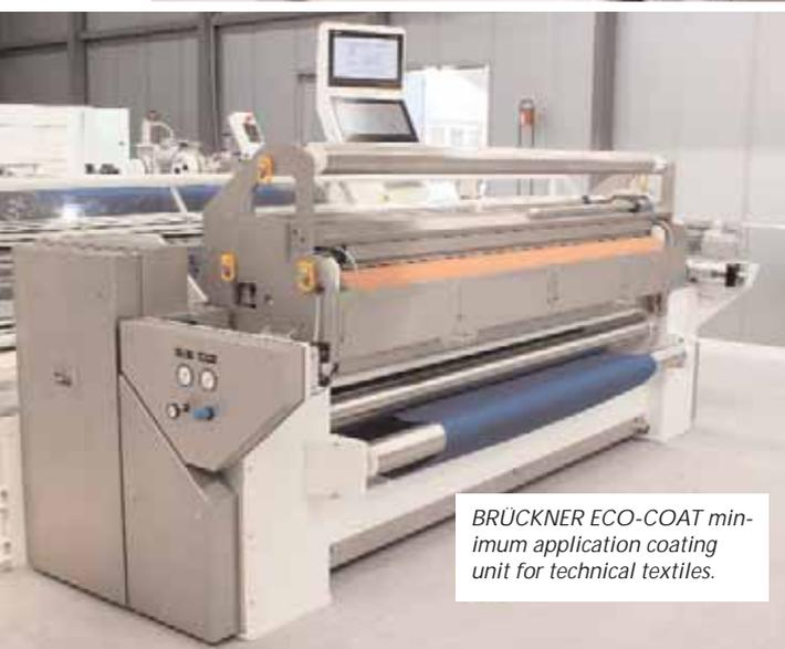
BRÜCKNER ECO-COAT minimum application coating unit for technical textiles.
