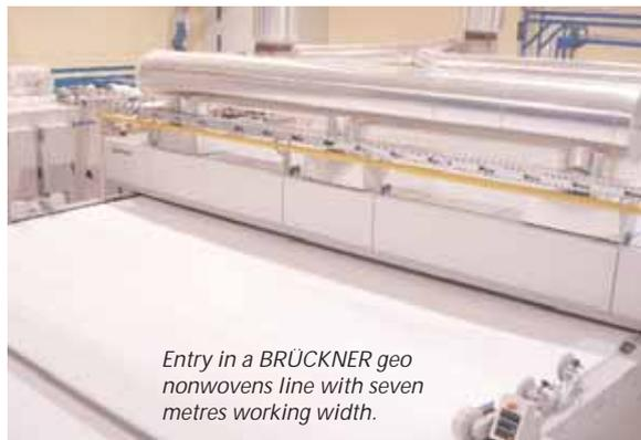
Entry in a BRÜCKNER geo nonwovens line with seven metres working width.
