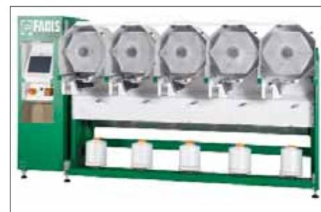
Thanks to this highly evolved technology, it is possible to process not only stretch polyamide yarns, but also all those elasticized yarns whose main prerogative is to maintain a high degree of residual elasticity after dyeing, such as Corespun yarns, covered elastomeric yarns, elasticized viscose, nylon PBT, polyester T400 and other similar yarns.
