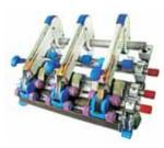
Dechang has recently launched the latest compact spinning technology suitable for 100% cotton, 100% viscose, PV, PC and various types of blends. It consists of longest drafting zone which
