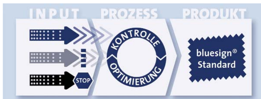
Diagram 1: Input Stream Management - critical substances are excluded right at the start of production
