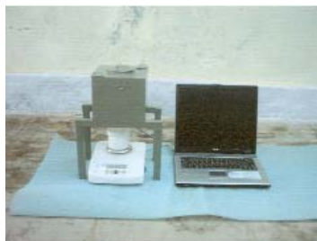
Fig 4. Water vapor resistance measuring Instrument with WVRTS Ver 1.1
